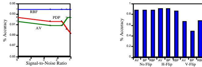
Figure 8. Comparison of various networks on noisy images (left) and image orientation (right).
